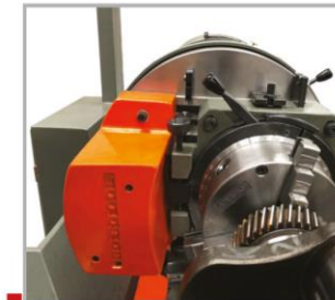
Dikey yatay hareketleri Strok kilitleri Horizontal and vertical movements tighten screws
